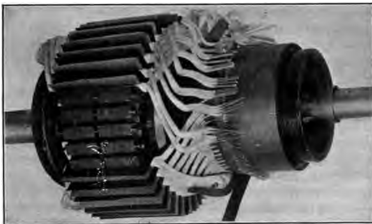
FIG. 107.—Armature partly wound showing insulation and method of connecting.
